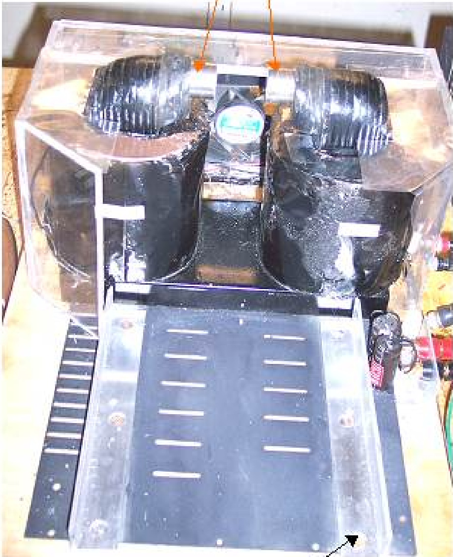
Poles for 2J21 magnetron (~1.2" gap)
